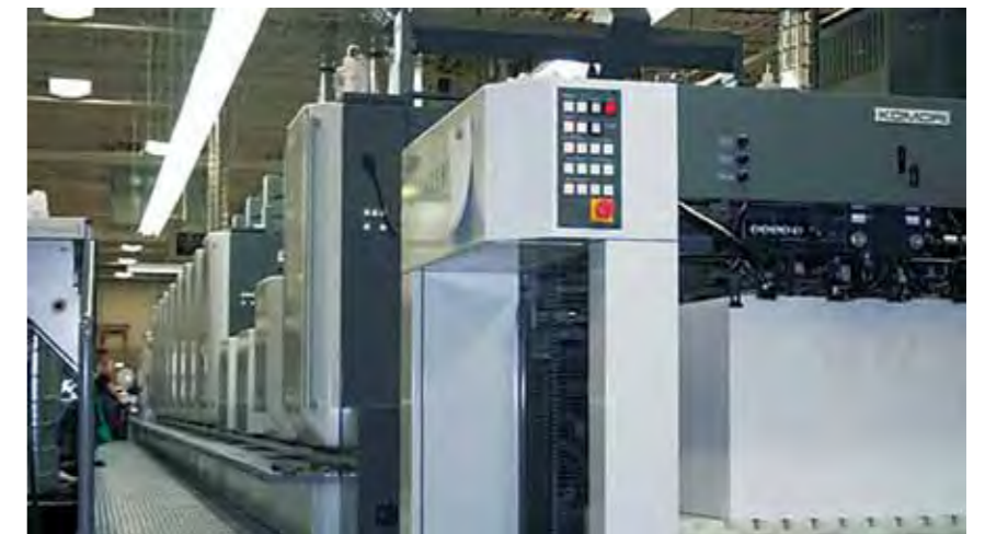
The specialty configuration UV press at Jones Packaging has two coaters, two drying units and nine printing units.
